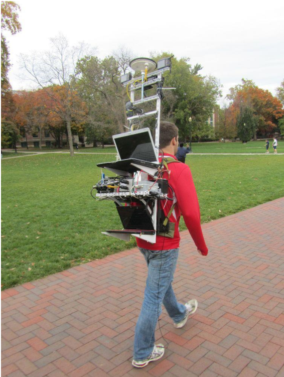
Figure 1. Sensor configuration in the portable navigator
