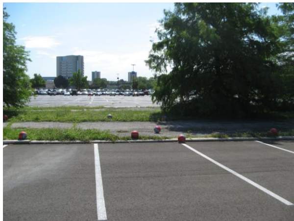
Figure 3. The field test: TLS data collection and the deployment of spherical targets (basketballs).
