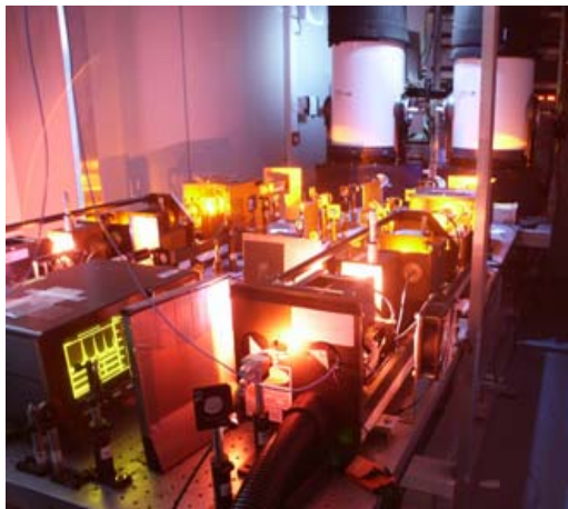
Fe-Boltzmann mobile lidar system deployed in Antarctica. Photo by Xinzhao Chu.
