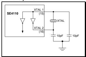
The PCB layout should avoid excessive track length between XTAL1 (Pin 15) and XTAL2 (Pin 16) and the crystal. The capacitors at each terminal of the crystal should be mounted adjacent to the crystal and have a low impedance connection to the ground plane in order to maintain the Oscillator Loop Gain and Phase-Noise performance under all conditions.
