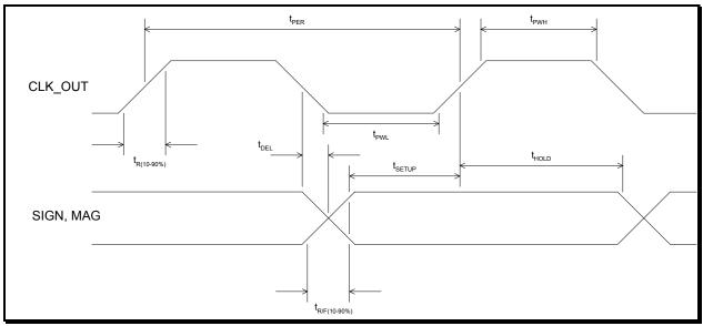
Conditions: C<sub>L</sub> ≤ 10 pF at Maximum Buffer Current
